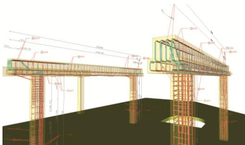
Figuur: Praktische wapening in Scia Engineer
