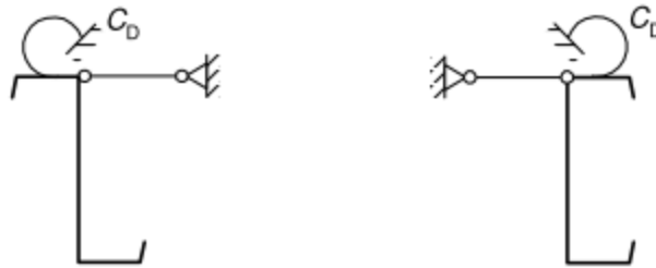
c) Model purlin as laterally braced with rotationally spring restraint C_D from sheeting
